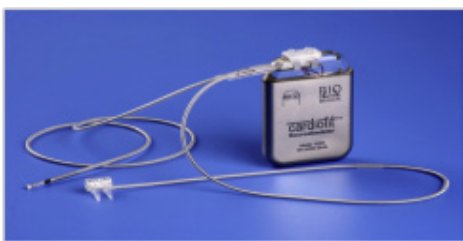
Figure 1: The CardioFit system. The CardioFit system consists of a stimulator, nerve stimulation lead with cuff and right ventricular sensing lead (28).
